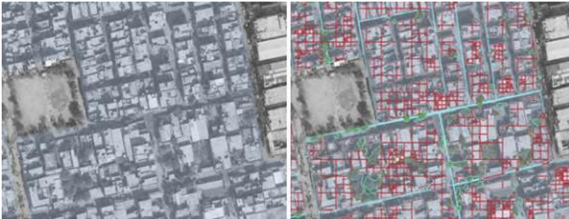
Figure 3. Example of quad-tree segmentation within built-up mask used for an estimation of area homogeneity indicator
